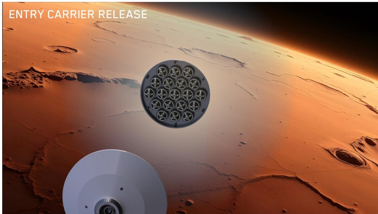
FIG. 1. Mars atmospheric entry. Artist's impression of small Mars atmospheric-entry vehicles carrying 19 probes behind a shared heat shield at the moment of backshell separation.
